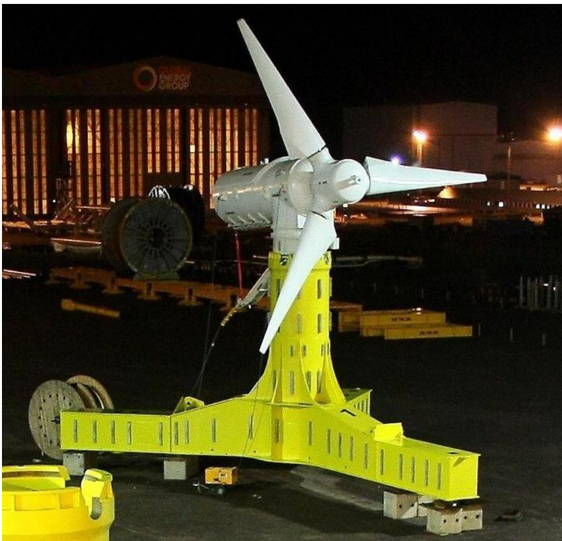
Figure 10 – AHH TTG sat atop a TSS onshore, note that no ballast is on the TSS
