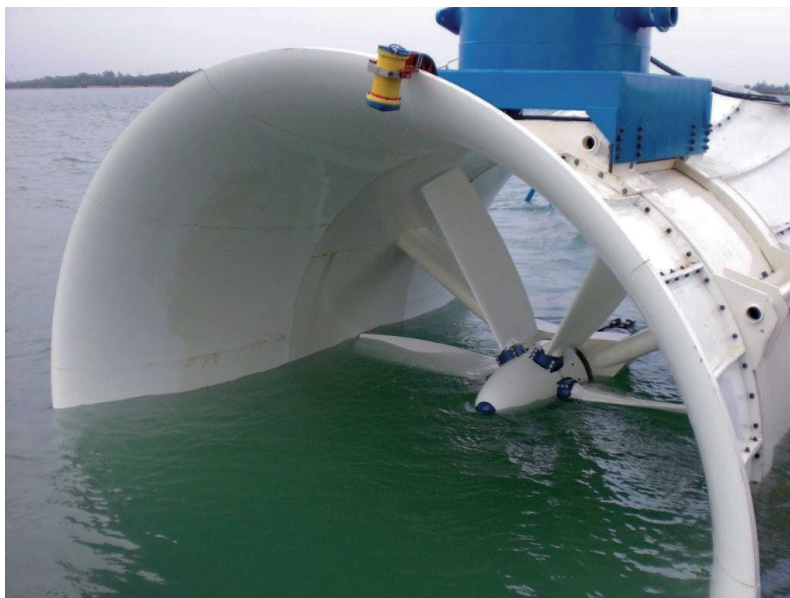
FIGURE 4.2 | SOLON TURBINE DURING TOW TESTING, SINGAPORE HARBOUR
