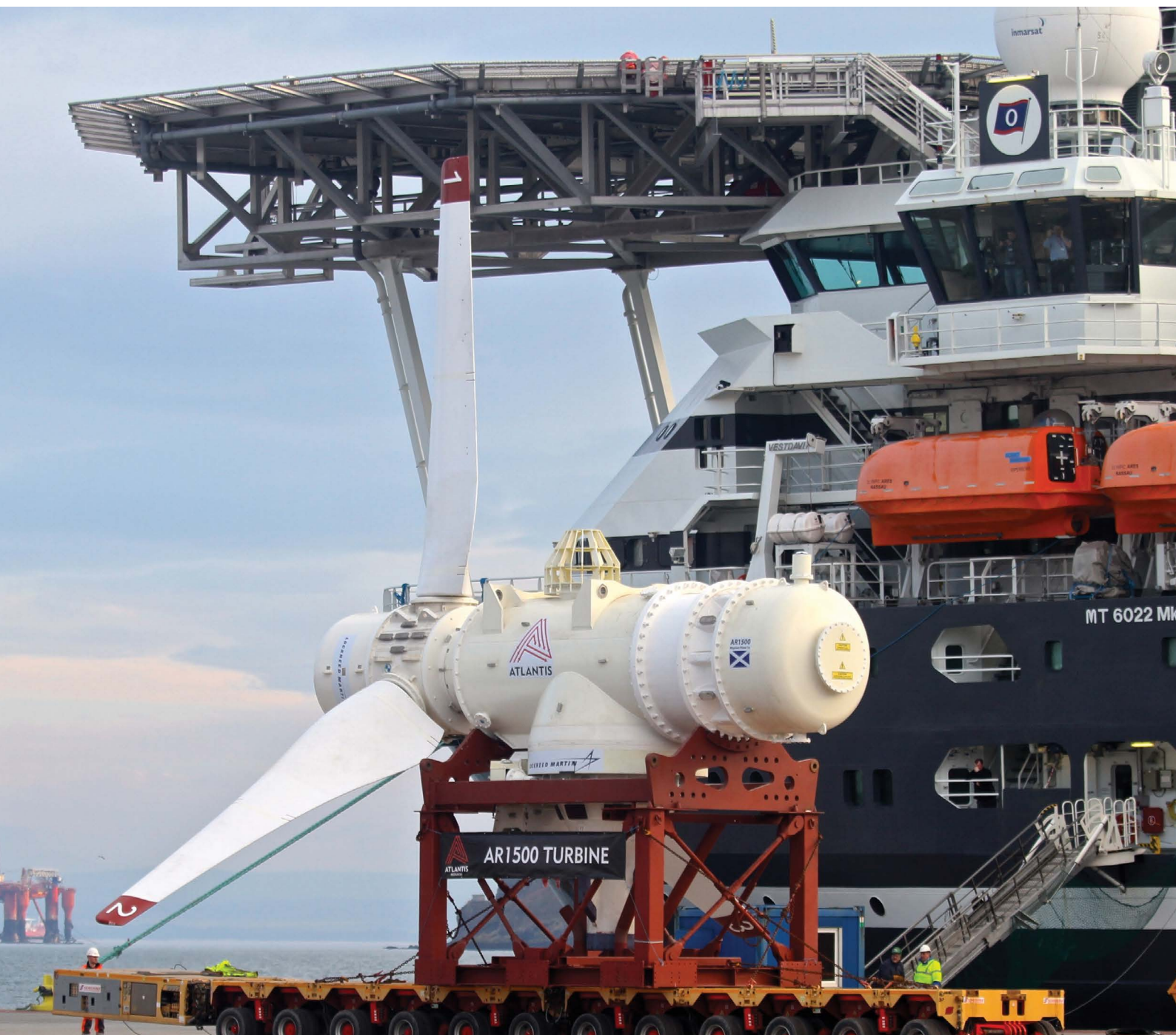
AR1500 1.5MW TURBINE READY TO BE LOADED OUT ONTO THE OLYMPIC ARES DP VESSEL
